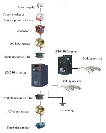
Fig.3-1 Connection of Inverter and Peripheral Devices
