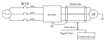
Fig.3-8 Solution to Inductive Interference
