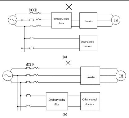
Fig. 3-6 Incorrect Installation of Noise Filter
