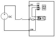
c: Use of external power supply in NPN mode d: Use of external power supply in PNP mode Fig. 3-14 Wiring Diagram of Multi-function Input Terminals
