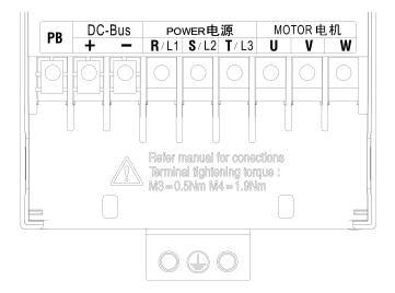
b) Schematic Diagram of Terminals (EM730-2R2-3B~EM730-4R0-3B)
