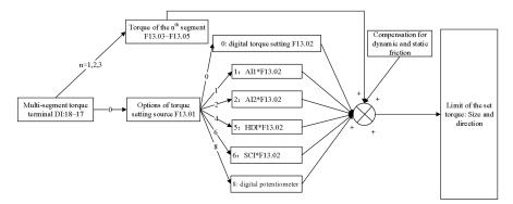
Fig. 1-5 Schematic Diagram of Torque Input Mode
