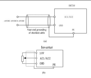
Fig.3-12 AI1/AI2 Terminal Wiring Diagram
