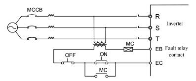
Fig.3-4 Connection of Input Circuit Breaker
