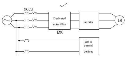
Fig.3-5 Correct Installation of Noise Filter
