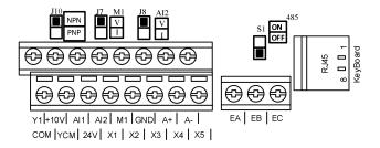
Fig.3-11 Layout of Control Circuit Terminals 1
