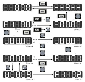
Fig. 4-4 Example of User-defined Mode Setting
