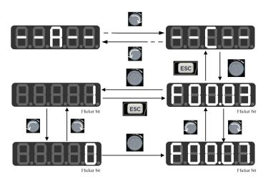
Fig. 4-5 Function Code Modification in Non-default Mode
