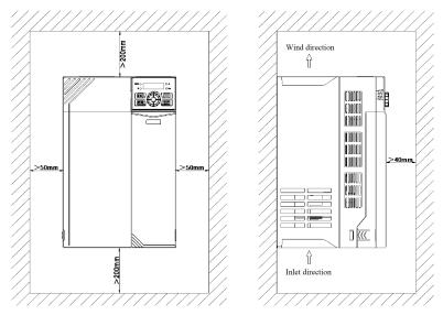
Fig.2-2 Inverter Installation Direction and Space
