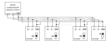
Fig. 3-17 Wiring of Communication Terminals of Multiple Inverters
