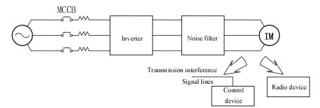
Fig.3-7 Noise Filter Installation on Output Side
